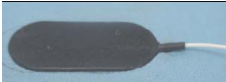
Fig. 1. Dry electrode made of conductive rubber and integrated into a garment with shielded cable
