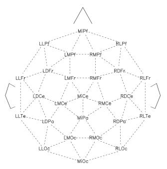
Figure 1. Schematic of the 26-electrode array used in the experiment.
